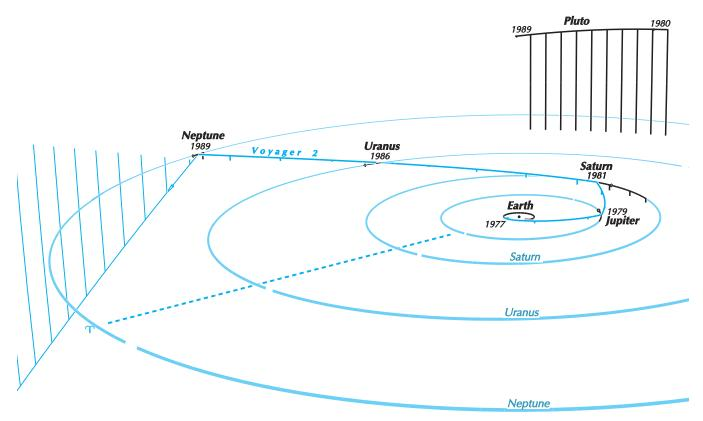
The Grand Curve. The four giant planets came into the lucky configuration in which each is behind the next one outward; this happens rarely, and soon ceases as the speedier inner planets overtake the outer ones. Thus each planet can "sling" a spacecraft toward the next.
